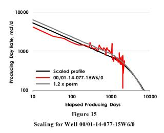
The scaled rates are slightly too low and should be adjusted by scaling the permeability thickness up by 20 percent.
