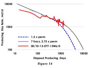
Alternate Scaling for Well 00/10-13-077-15W6/0
