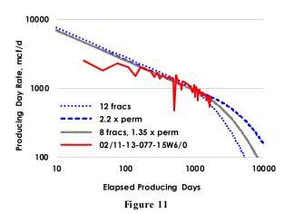
Alternate Scaling for Well 00/05-13-077-15W6/0
